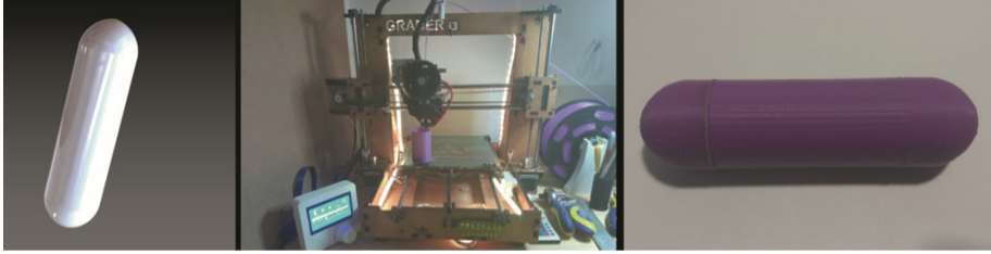
Fig. 2. 3D model of the sex toy plastic body, 3D printing of the parts and the plastic body assembled.
