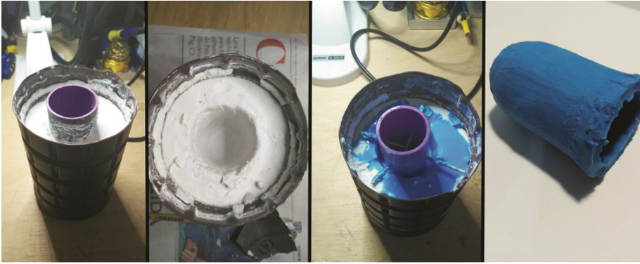
Fig. 6. The silicone casting process for creating the sleeve of the sex toy.
